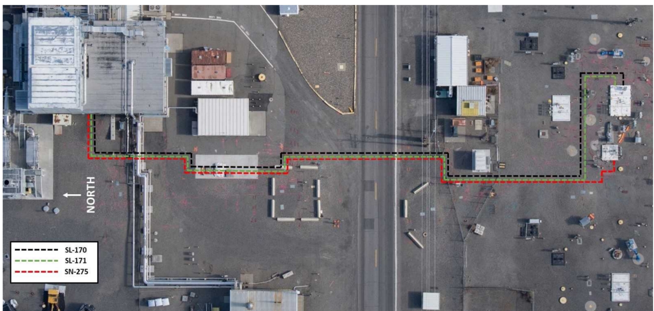
Figure 1: Evaporator to AW-Farm Transfer Line Layout
