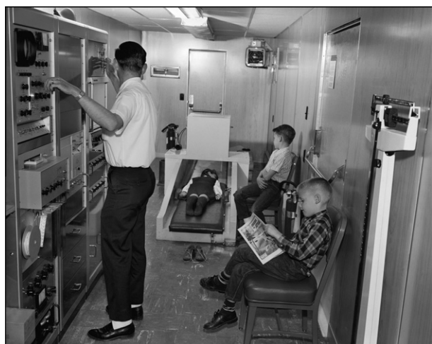
Fig. 10. This 1965 photograph records the inside of a truck-mounted whole-body radiation counter hauled to schools to monitor radiation levels in children (US Department of Energy).
