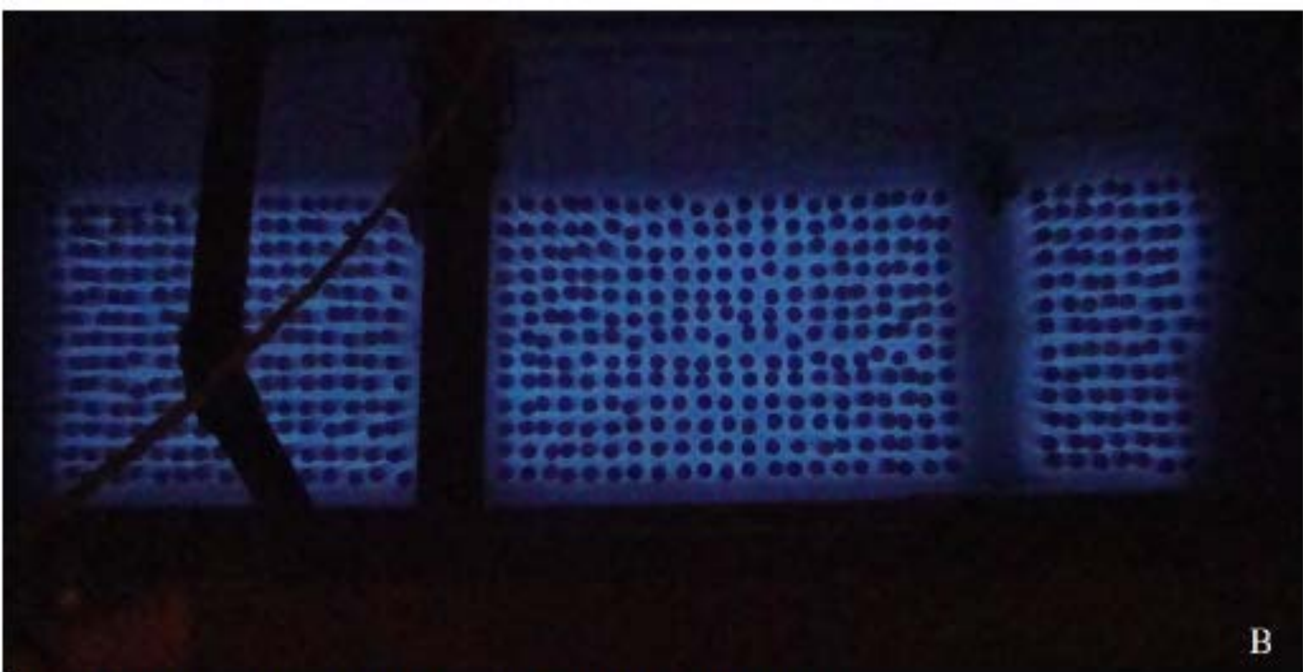
Figure 13 - Cherenkov radiation glow: A) Cell 6. B) Cell 7.
