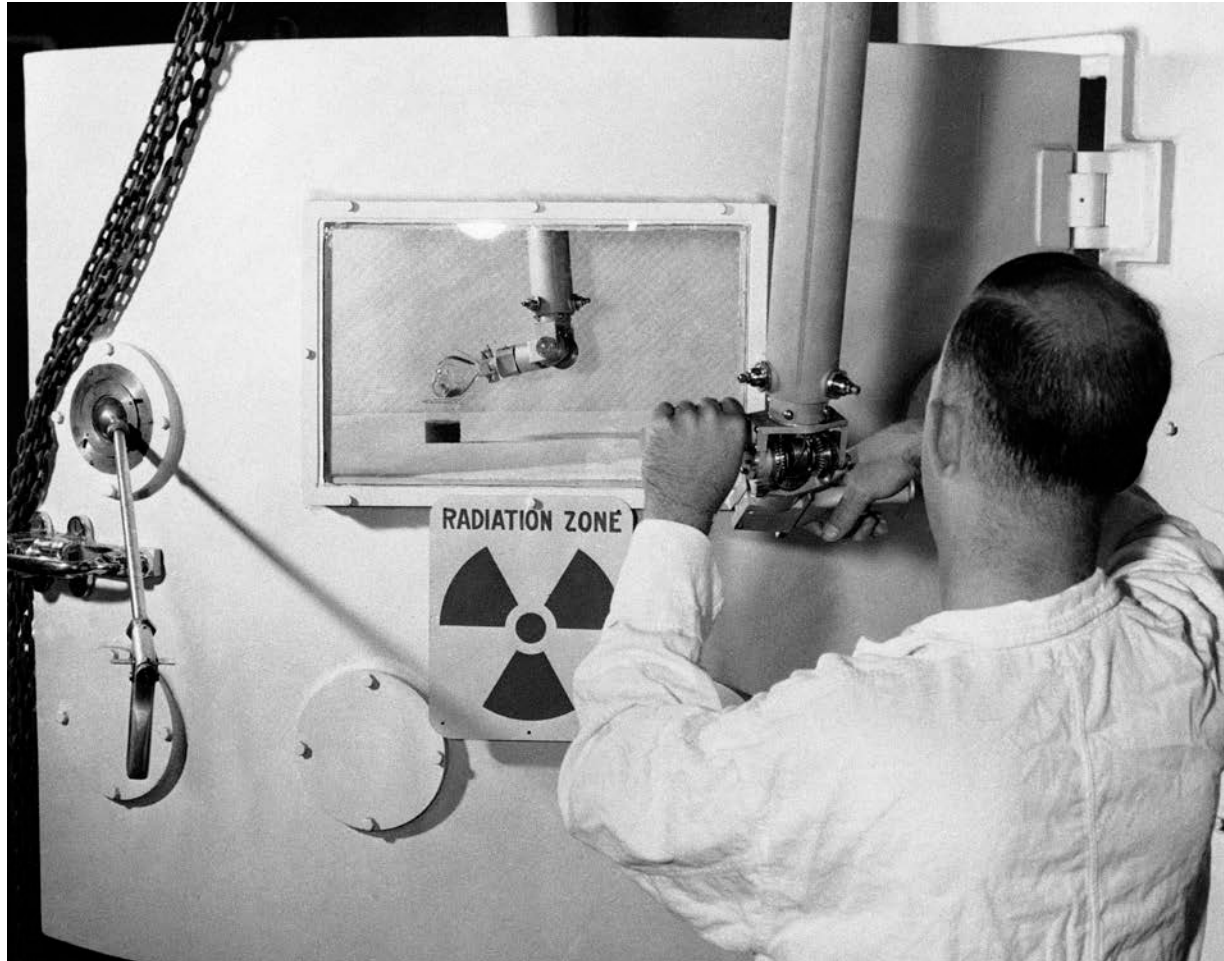
An operator works a mechanical hand on the other side of a protective wall at the Hanford atomic energy plant in Richland, July 31, 1954. (AP)
