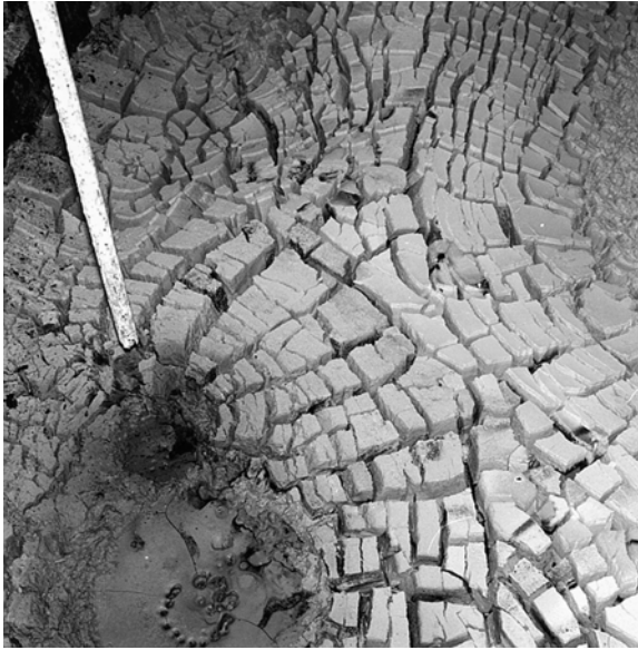
Figure 4: Diatomaceous earth in Hanford Tank 104-U (capacity, 530,000 gallons). (Source: Pacific Northwest National Laboratory.)
